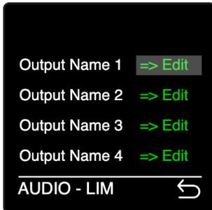
To adjust a limiter, select and press => **Edit** on the channel you want to adjust
