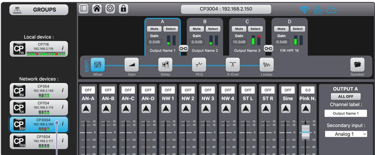
When you select another MPA / DA series™ amplifier within the network, its USER interface will be displayed, allowing you to operate it.
