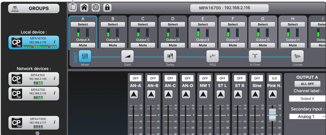
The sidebar displays the currently connected device as the "Local device," and it lists other MPA / DA series™ amplifiers in the network as "Network devices."
