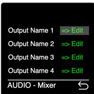
To edit a mixing matrix, select and press => **Edit** on the channel you want to adjust.
