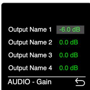
To edit a **gain** value, select the channel you wish to edit and press the dB value to control it. Turn the rotary to increase or decrease the value and press again to confirm.
