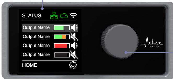
All controls are performed using a single **rotary encoder**. Rotate the encoder to navigate through the menus. Pressing the rotary controller inwards executes an **ENTER** action.
