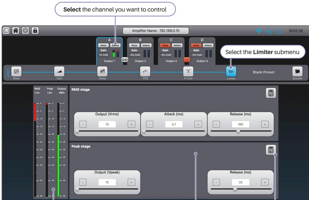
The **red meters** show the selected channel's RMS and Peak gain reduction in dB, while the **green meter** displays the output level after limiting in dBFS.
