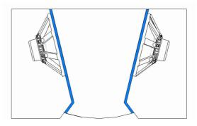
The double interactive load provides excellent control of transducer displacement, which significantly increases mechanical reliability.
