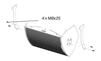
2. Assemble by approaching the iX12 under the iS115 then fix the junction pieces to the iS115 using the M8x25 screws.
