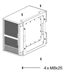
2. If necessary, it is possible to fix the assembly on a section of wall using the fixing holes.
