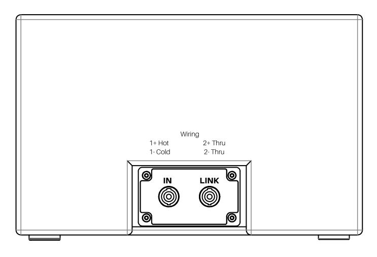
The rear panel of the iS Series subwoofers are equipped with two NL4 connectors. The four pins of the two connectors are connected in parallel. The speakers occupy points 1 + / 1-.
