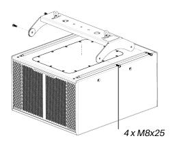
2. Use the lifting rings to suspend and secure the subwoofer with a motor for example.
