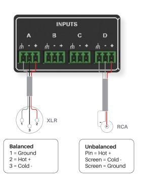
Terminal block connector for REMOTE applications, EN-54 ready.
