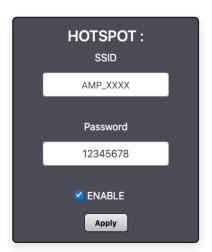
Activate the **Hotspot** by ticking the checkbox. Then search for the **SSID** name within your device's available Wi-Fi networks. Connect to the hotspot and enter IP address **172.24.0.1** in your browser's URL. This will automatically open the IntelliCloud web interface on your device.
