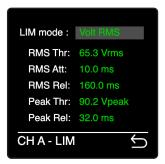
**LIM mode:** enables you to set the limiter manually by adjusting the Vrms threshold, or allows the MPA / DA series to calculate a setting based on the impedance and wattage of your speaker. To achieve this, select the preset that has the same Ohm value as the connected speaker, and then set the correct Wrms and Wpeak values in the controls below.
