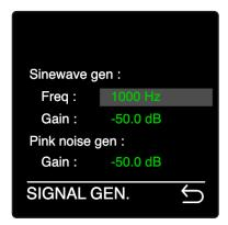
You have access to both a pink noise and a sine wave generator with eight selectable frequencies: 50, 100, 200, 500, 1000, 2000, 5000, or 10000 Hz. The level for the sine wave can be adjusted within the range of -50 dB to -20 dB, while the pink noise level can be adjusted within the range of -50 dB to -10 dB.
