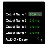
To edit a **delay** time, select the channel you wish to edit and press the ms value to control it. Turn the rotary to increase or decrease the value and press again to confirm.
