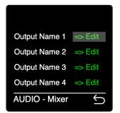
To edit a mixing matrix, select and press => Edit on the channel you want to adjust.
