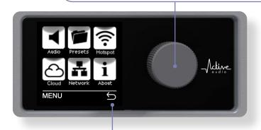
Select and press the **return icon**  $\subseteq$  to navigate back one level in the menu and return to the hompage.
