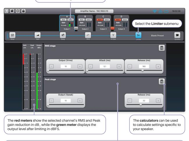
**Output (Vrms)** and **(Vpeak)** serve as **threshold** controls that determine the signal level at which the limiter engages. These thresholds can be adjusted within the range of -56 to +24 dBu.
