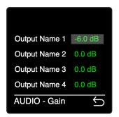
To edit a **gain** value, select the channel you wish to edit and press the dB value to control it. Turn the rotary to increase or decrease the value and press again to again to confirm.
