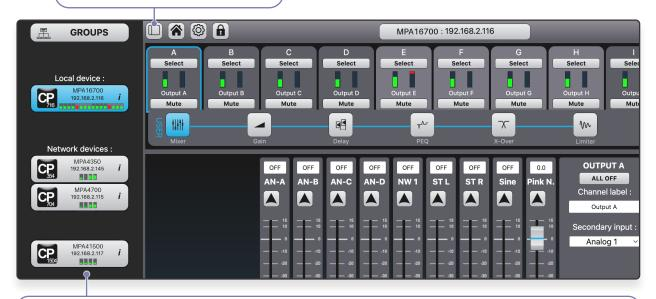
The sidebar displays the currently connected device as the "Local device," and it lists other MPA / DA series™ amplifiers in the network as "Network devices."
