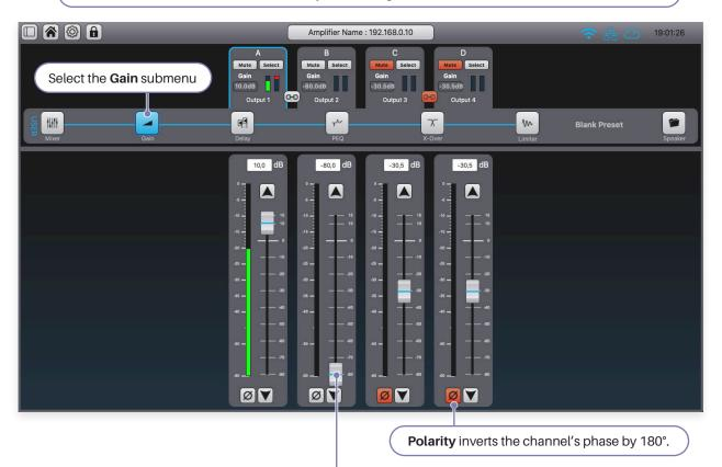
Adjust the faders to reach the desired output volume.
