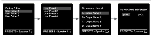
To insert a speaker preset onto a channel: Select a speaker preset folder > Select a preset > Select the channel on which you wish to load the preset > And finally, press YES to confirm your choice and insert the preset.
