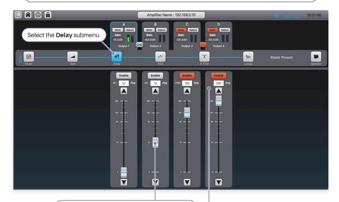
Set the desired **delay time** for each channel using the fader, arrows, keyboard, or input field. Double-click on the fader to reset it to 0 ms.
