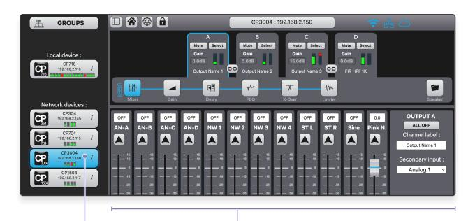
When you select another MPA / DA series™ amplifier within the network, its USER interface will be displayed, allowing you to operate it.
