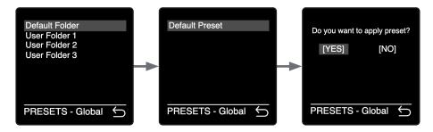
To recall a global preset: Select a global preset folder > Select a preset to load > And finally, press YES to confirm your choice and load the preset.
