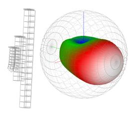
Playing with arrays lengths to match directivity thru the whole spectrum
