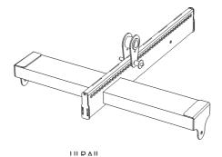
The ULRAIL lifting/flying accessory stands for the perfect alternative to ULTRUSS, for hanging small clusters. It permits to hang up to 6 UL210 or UL210D speakers, for a maximum weight of 250 kg (550 lbs).
