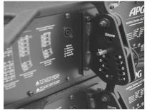
Angle setup on the back before lifting: one man setup
