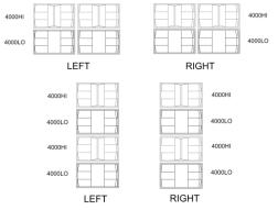
The two possible configurations with a standard Matrix Array kit.
