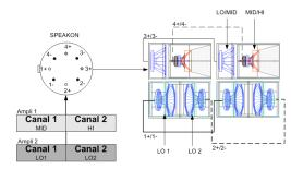
"Loudspeaker" internal wiring
