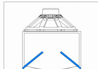
The double interactive load provides excellent control of transducer displacement, which significantly increases mechanical reliability.
