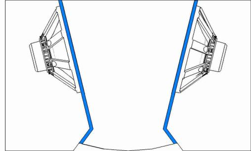
The double interactive load provides excellent control of transducer displacement, which significantly increases mechanical reliability.
